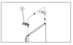
Pull upper bearing block (a) out, and replace it on the opposite side.
